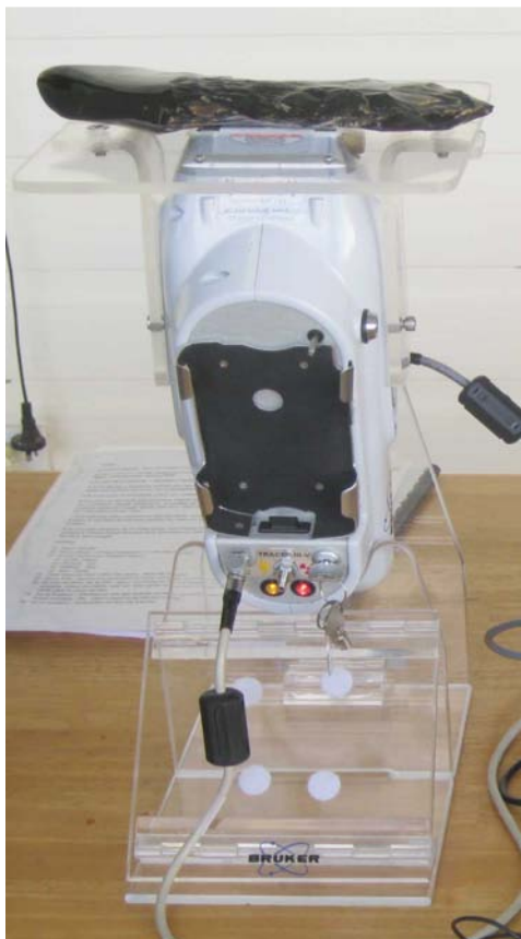
Figure 4. A large obsidian artefact placed on a large stage purpose-built for the Bruker Tracer III-IV PXRf (photo by Peter White)
