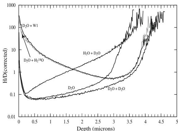
Fig. 8. H/D ratios in the five experiments in which D<sub>2</sub>O was used. Each curve is labeled with the fluid used for each half of the reaction in the order in which they were run.
