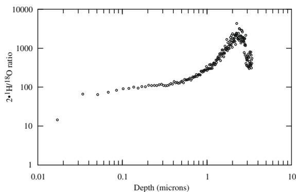
Fig. 10. Hydrogen to oxygen ratio in the hydration profile of the experiment run for 5 days in  $\text{H}_2^{18}\text{O}$ . Data are plotted as  $2 \cdot \text{H}/^{18}\text{O}$ .
