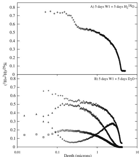
Fig. 3. Ten-day isotope exchange experiments in which water W1 was used for the first 5 days of the experiment. Squares: uncorrected D/<sup>29</sup>Si, Triangles: corrected D/<sup>29</sup>Si, Diamonds H/<sup>29</sup>Si, Circles: (H + D)/<sup>29</sup>Si. (A) Five days in water W1 followed by 5 days in H<sub>2</sub><sup>18</sup>O. (B) Five days in water W1 followed by 5 days in D<sub>2</sub>O. All experiments were conducted at 150 °C at a pressure on the liquid–vapor curve.
