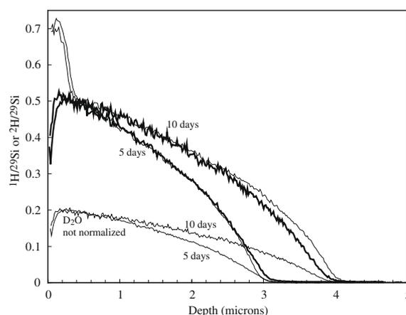
Fig. 2. Original and corrected 5- and 10-day deuterium profiles compared to hydrogen profiles run for identical times, showing the effect of correction for differential ionization efficiencies. Heavy lines: normalized D<sub>2</sub>O values.
