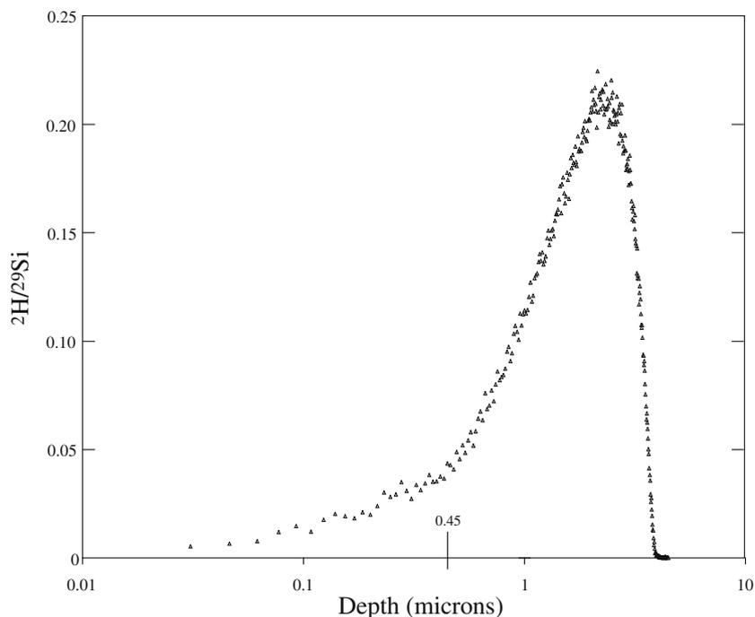
Fig. 7. Intensity-corrected D<sub>2</sub>O depth profile for the experiment run for 5 days in D<sub>2</sub>O followed by 5 days in H<sub>2</sub><sup>18</sup>O. Note the change in slope in the profile near 0.45 μm.
