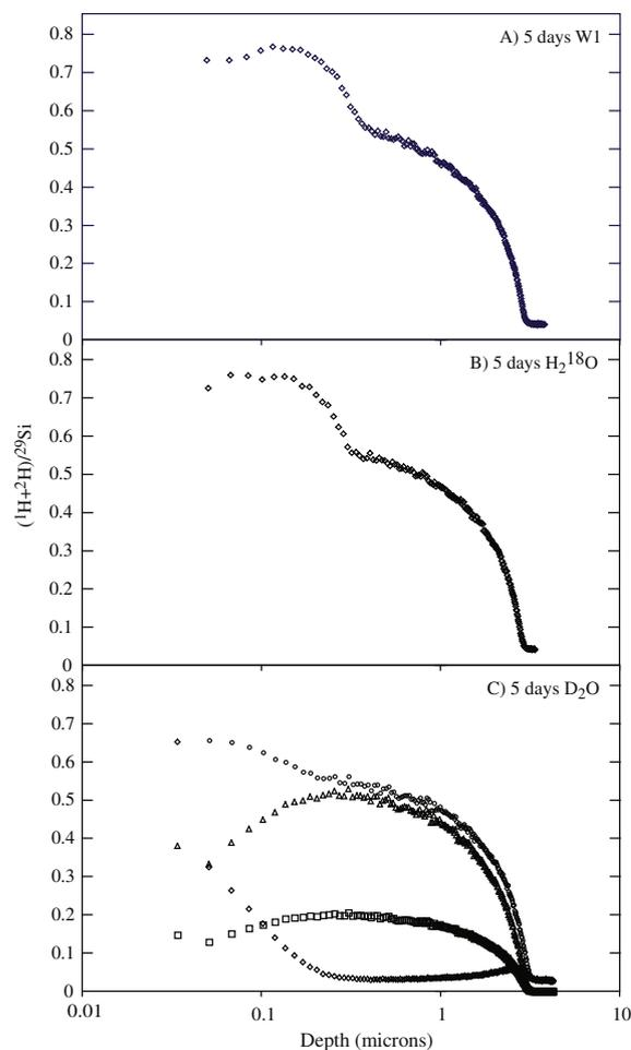
Fig. 5. Five-day, single-isotope experiments. Squares: uncorrected D/<sup>29</sup>Si, Triangles: corrected D/<sup>29</sup>Si, Diamonds H/<sup>29</sup>Si, Circles: (H+D)/<sup>29</sup>Si. (A) Five days in water W1. (B) Five days in water H<sub>2</sub><sup>18</sup>O. (C) Five days in D<sub>2</sub>O. All experiments were conducted at 150 °C at a pressure on the liquid–vapor curve.
