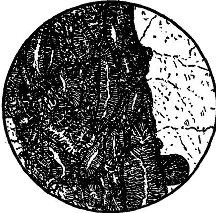
In the upper part of the field is a large glassy fragment, on the margin of which a thin spherulitic envelope has developed. The main part of the field is occupied by smaller fragments of glass, which have also become devitrified from their outer surfaces inwards.
