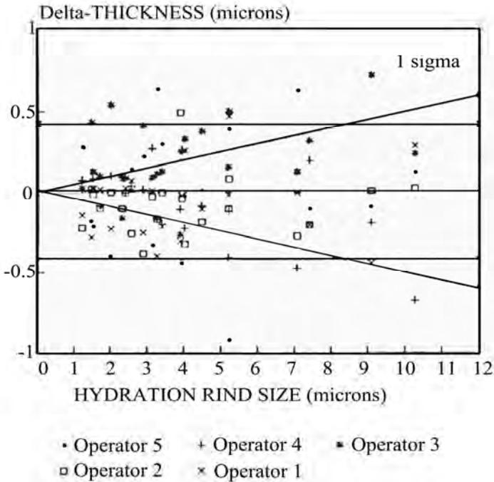
**Figure 1.** Delta-T vs. Rind Thickness, aggregate for all observers. Resolution limit +/- 0.5 $\mu$ m, based on 550nm “green”.
