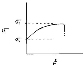
Fig. 1 Hypothetical curve of stress ( $\sigma$ ) versus rate of strain ( $\dot{\epsilon}$ ) for lava possessing yield strength ( $\sigma_y$ ), tensile strength ( $\sigma_t$ ), and pseudoplastic behavior. Brittle failure occurs when stress reaches tensile strength (from [16])
