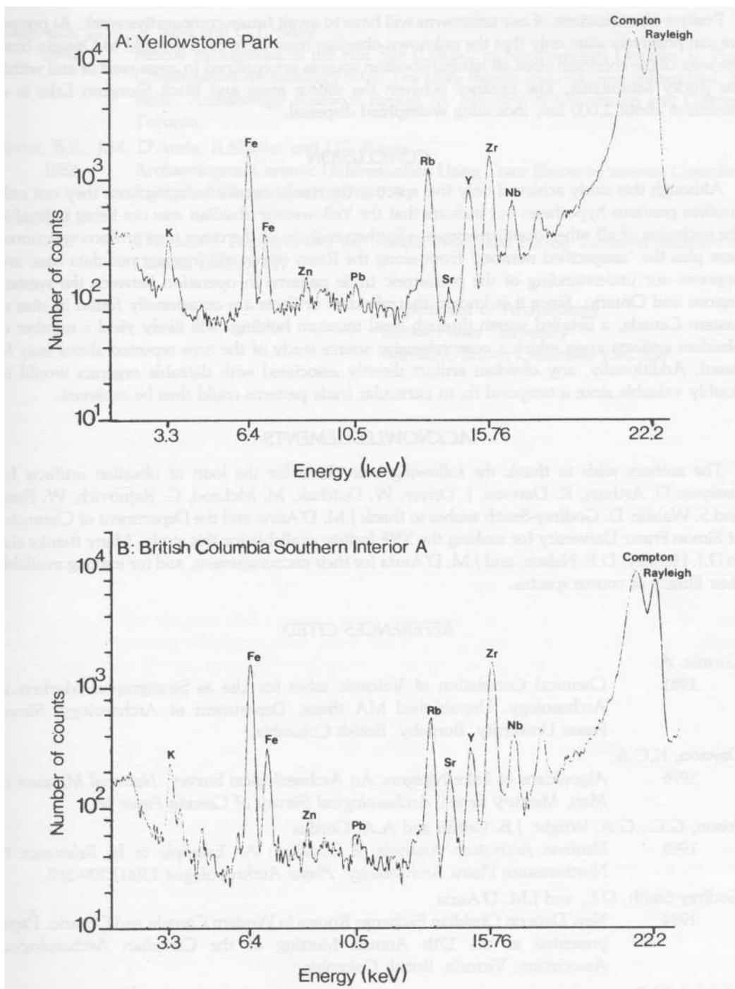
Fig. 2: XRF spectra of the artifacts analyzed.
