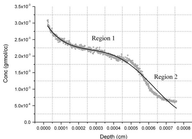
**Figure 6.** SIMS profile of YAL-2 sample (points) and the 3rd order fitting polynomial (line) with  $Rsq = 0.98$ . Diffusion regions 1 & 2 are indicated (see text).
