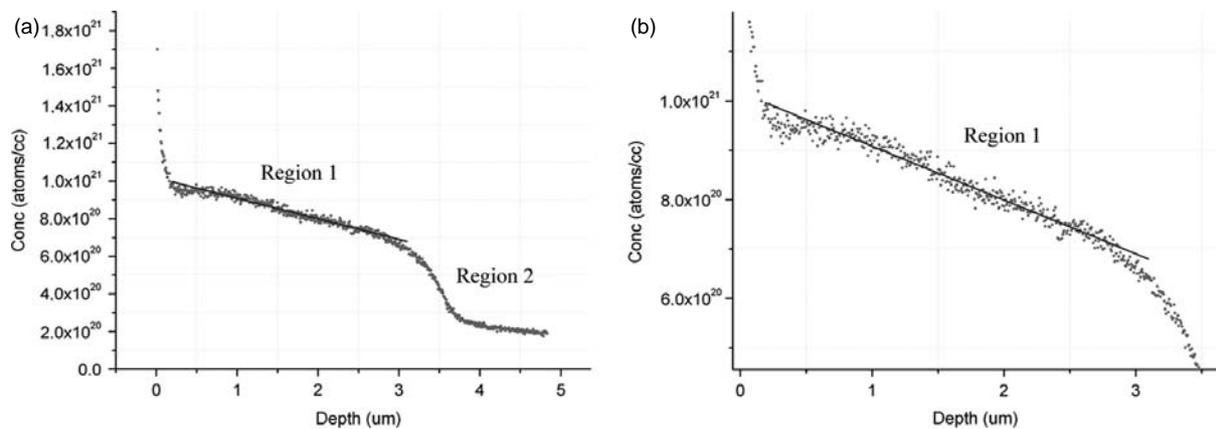
**Figure 3.** (a) SIMS profile of YR-2 from Yali island, with the linear regression in the diffused region and (b) a more detailed image of the diffused region, Diffusion regions 1 and 2, are shown (see text).
