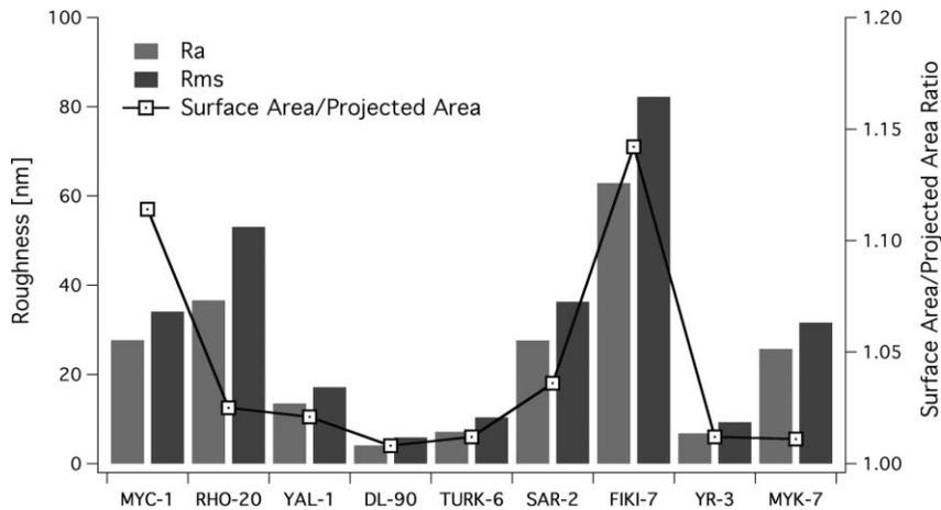
**Figure 2.** Roughness (Ra, Rms) in nm and Area ratios factor for all examined samples.
