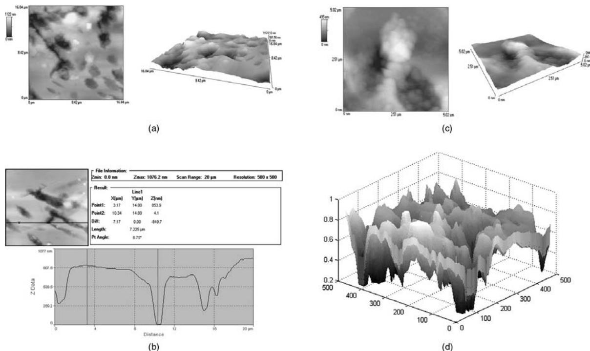
**Figure 1.** (a) Topography image (left) and its three-dimensional representation (right) of a  $16.84 \times 16.84 \mu\text{m}$  spot of the MYC sample, (b) Line profile analysis of a  $20.00 \times 20.00 \mu\text{m}$  spot of the MYC sample, (c) Topography image (left) and its three-dimensional representation (right) of a  $5.02 \times 5.02 \mu\text{m}$  spot of the MYC sample (d) 3D representation of Fig. 1(a) (left). The x and y axis are pixels and z is colour scale.
